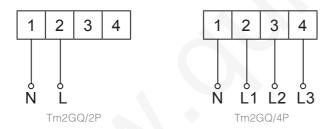
Note: L and N wiring cannot be reversed
