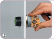
Buckle the switching elements directly. The actuator symbol can be installed directly in the front (normally, it has been installed before out of the factory). When the illuminated pushbutton is installed, buckle the lampholder first and switching elements successively. Note: after installation, check if the buckle of the switching elements is completely locked.
