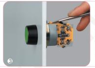
Remove the switching elements or lampholder: remove the locked assemblies freely and easily by lifting the buckle of the locking system with a screwdriver.
