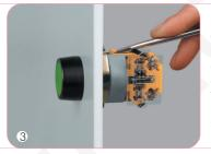
Remove the switching elements or lampholder: remove the locked assemblies freely and easily by lifting the buckle of the locking system with a screwdriver.
