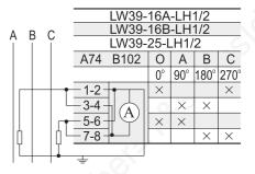
3 transformers, with N line, changeover measurement A, B, C, N 3-phase 4-wire current
