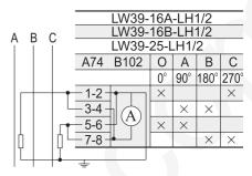
3 transformers, with N line, changeover measurement A, B, C, N 3-phase 4-wire current
