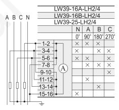
3 transformers, with "0" position, changeover measurement A, B, C 3-phase current
