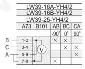
With "0" position, N line, 3-phase phase voltage and 3-phasse wire voltage of changeover measurement
