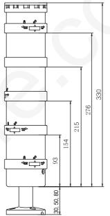
Dimension (4 optical elements + 1 acoustic element)
