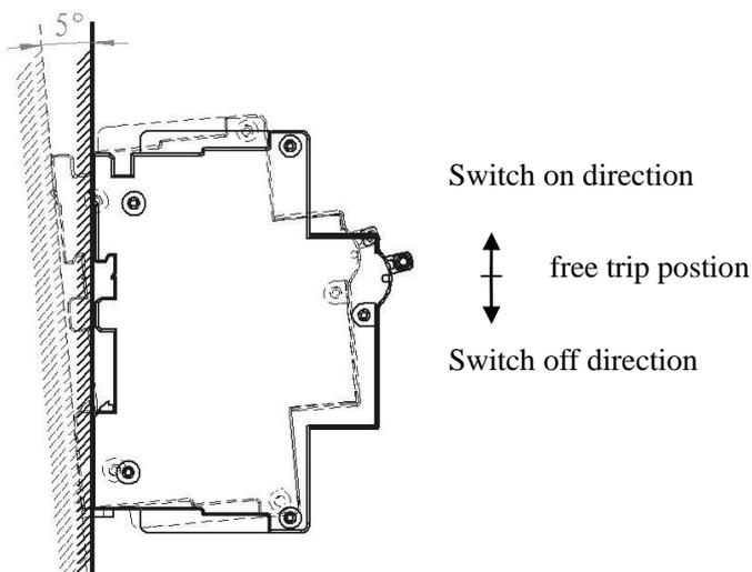
**DIN Rail Installation.** The breaker should be mounted within 5° of the mounting plane in case the characters of the product are affected.
