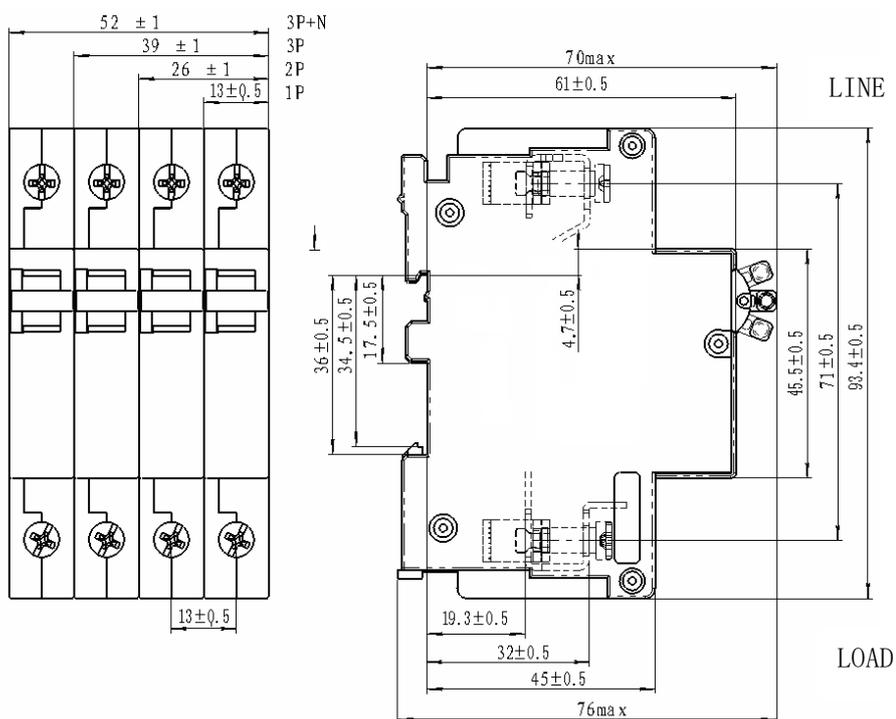
**2) Configuration & Installation Dimension of the product with 57mm operation face**
