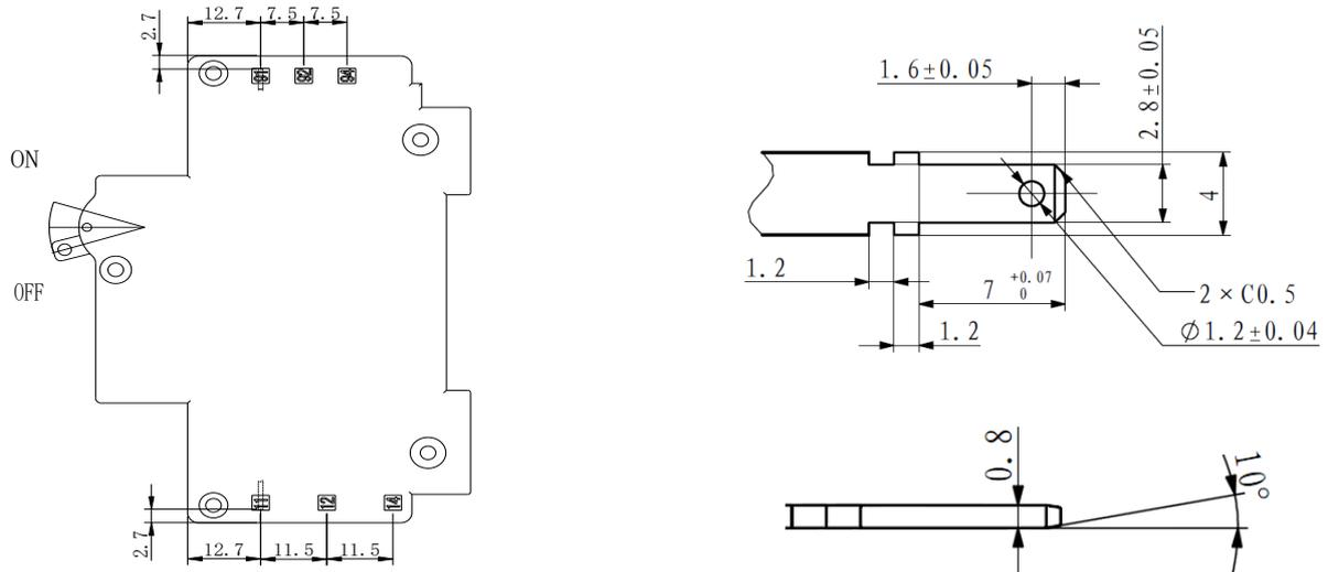
10.2 NDB5 series HMCB can attach only one pair of auxiliary signal function, which terminal is pluggable connection strap.
