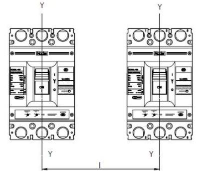
Note: Check the connected busbar or cable during rowing or stacking ensure that the air insulation distance won't be reduced.
