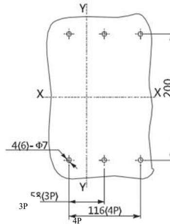
Note: The limit deviation not indicated with the tolerance dimensions is as per GB/T 1804-m.
